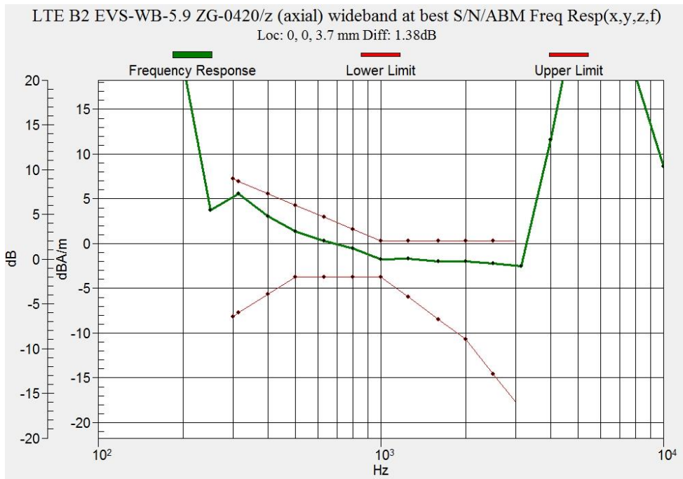
Figure B.4 Frequency Response of LTE Band 2
