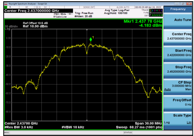
Power spectral density-802.11g ,2412MHz,Ant0
