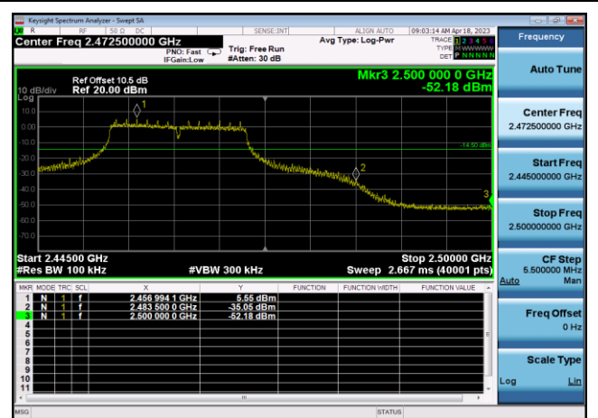
,Plot 2,Band Edge-802.11g,2462MHz ,Ant0
