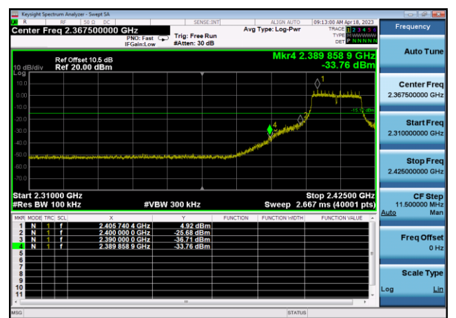
,Plot 2,Band Edge-802.11g,2462MHz ,Ant0
