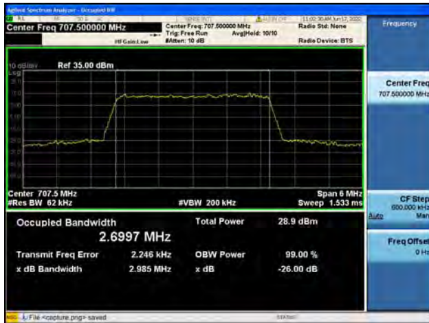
B12 / 3MHz / QPSK/ High CH
