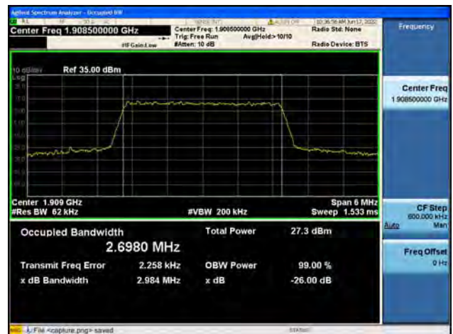
B2 / 3MHz / 16QAM/ High CH
