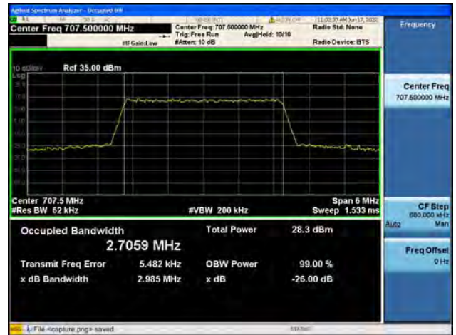
B12 / 3MHz / 16QAM/ High CH
