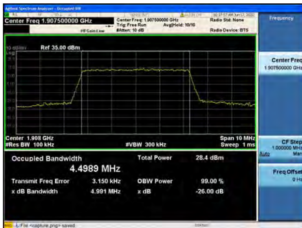
B2 / 5MHz / QPSK/ High CH
