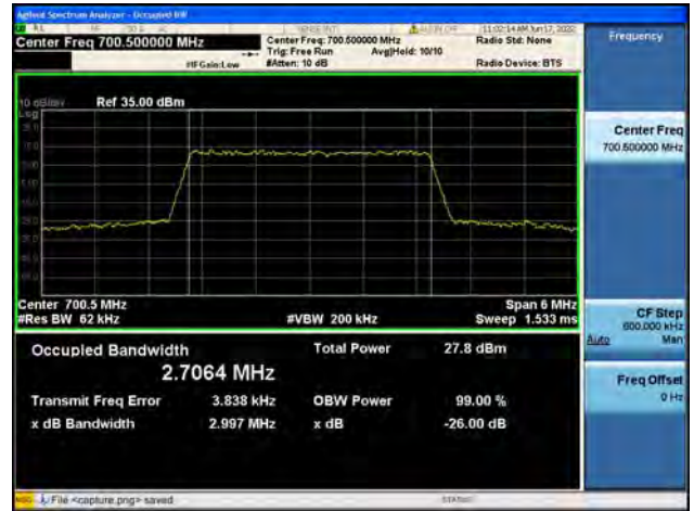
B12 / 3MHz / 16QAM/ Mid CH
