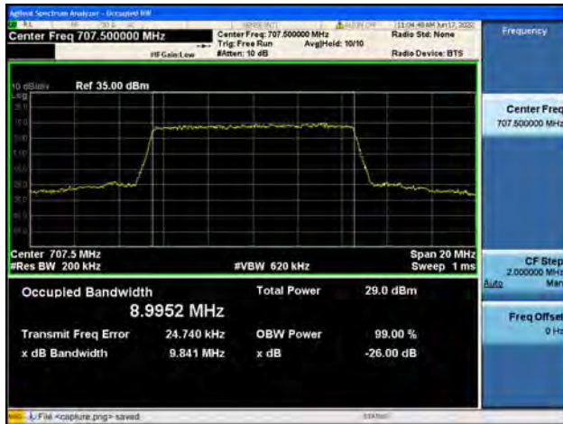
B12 / 10MHz / QPSK/ High CH
