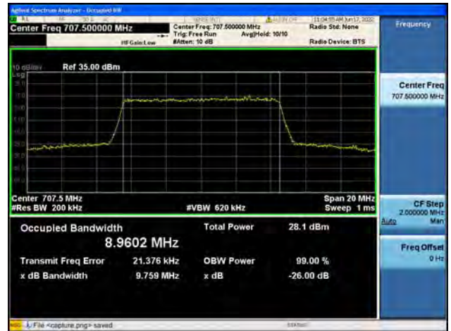
B12 / 10MHz / 16QAM/ High CH
