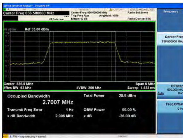
B5 / 3MHz / QPSK/ High CH
