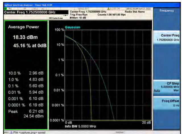
B4 / 5MHz / High CH / 16QAM
