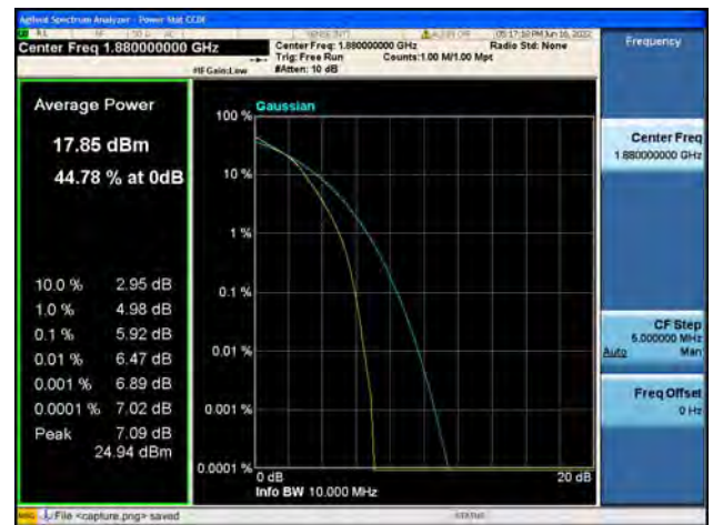
B2 / 10MHz / High CH / 16QAM
