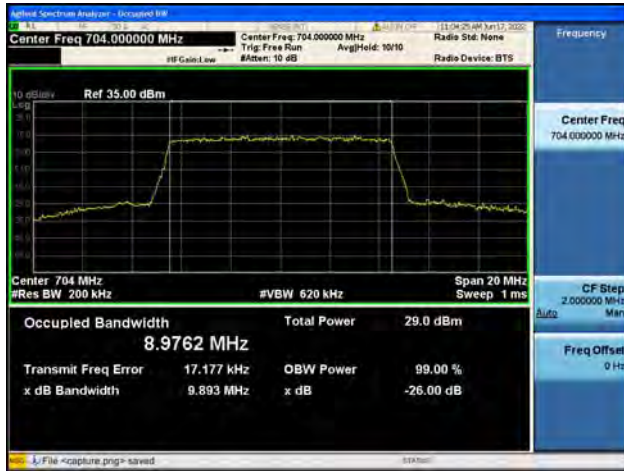
B12 / 10MHz / QPSK/ Mid CH
