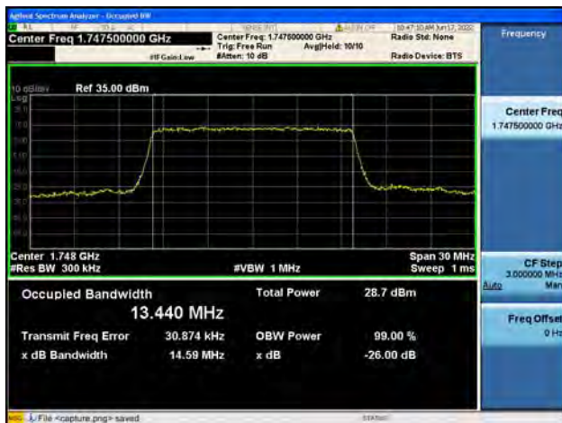
B4 / 15MHz / QPSK/ High CH
