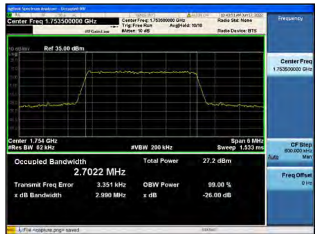
B4 / 3MHz / 16QAM/ High CH
