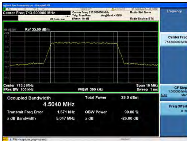
B12 / 5MHz / QPSK/ High CH
