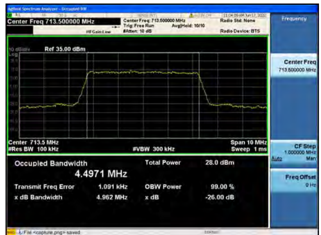
B12 / 5MHz / 16QAM/ High CH
