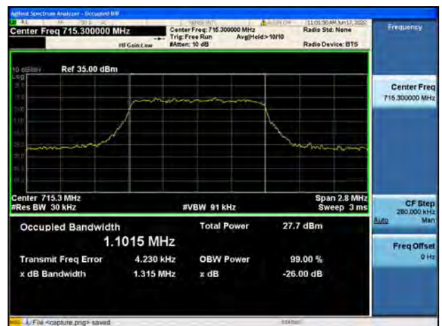
B12 / 1.4MHz / 16QAM/ High CH
