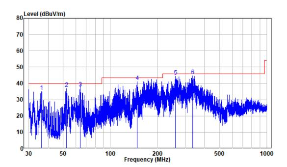
Site : chamber Condition: 3m VERTICAL Job No. : SZNS1220402-12303E-EM Test Mode: Lighting
