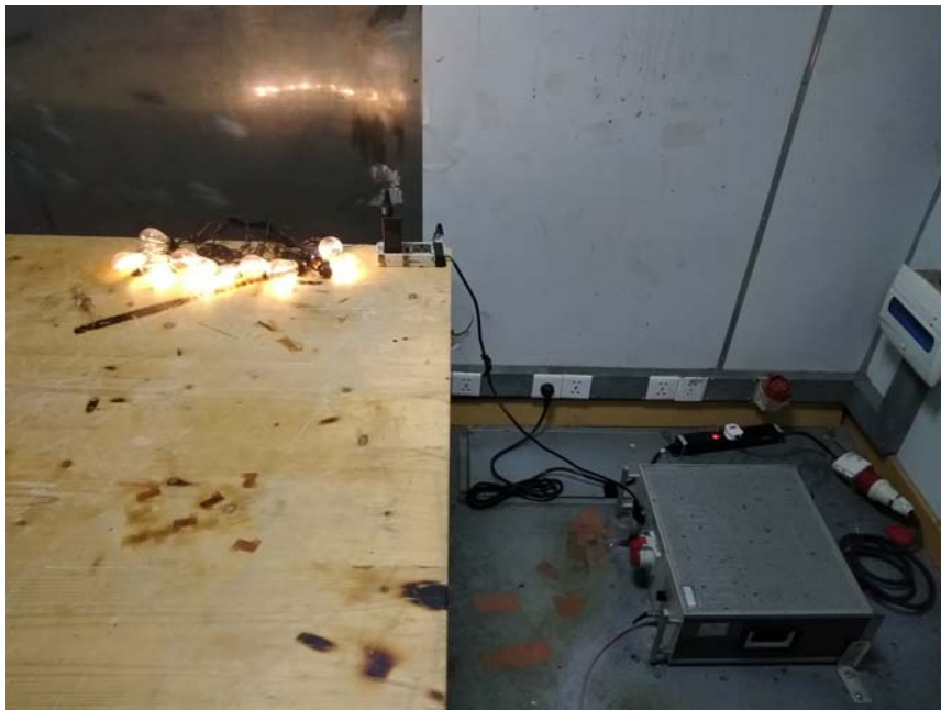
Photograph of set-up for conducted Emission
