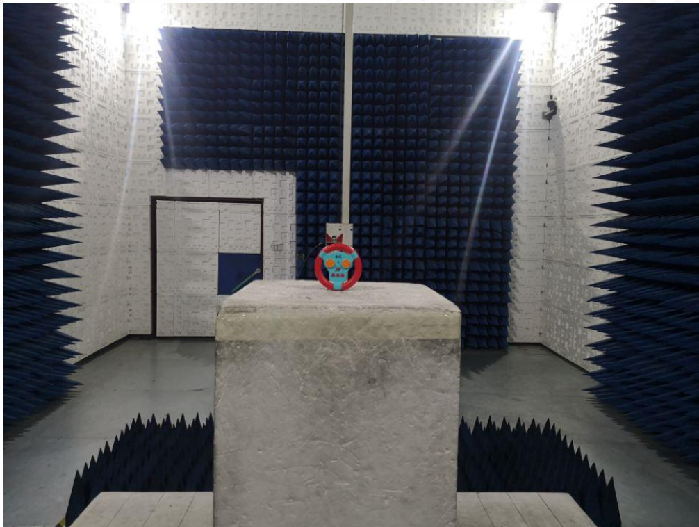
RADIATED EMISSION TEST SETUP ABOVE 1GHZ
