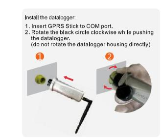
The device must be installed away from the strong **Delivery Content** magnetic field produced by large electrical appliances ■ 1 GPRS stick such as microwave oven, refrigerator, telephone, metal 1 GPRS Antenna walls,etc.Otherwise, the communication quality may be affected. It may also be affected by lighting storm. 1 Quick Installation Manual
