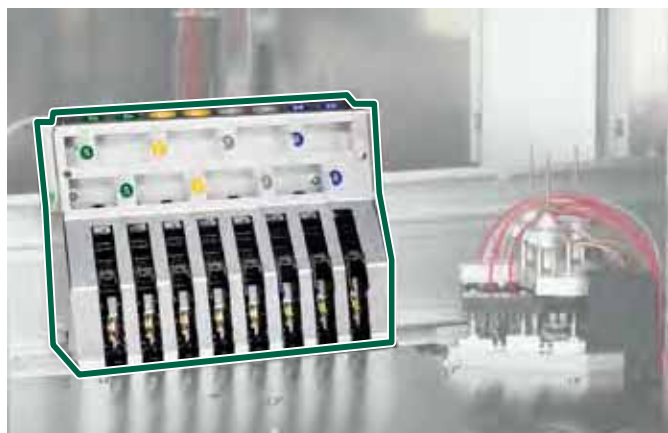
(reagent carriage localization - reagent door opened)
