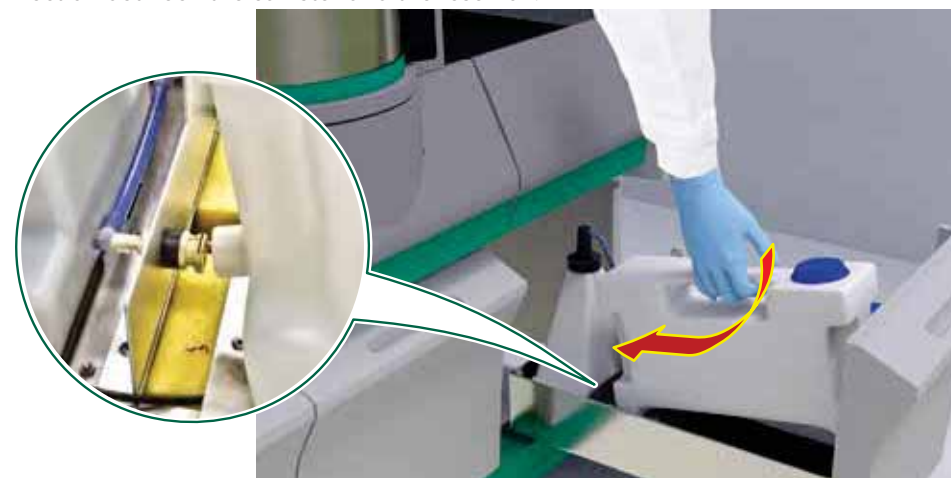
(loading of the water canister, mind the water canister / reservoir connection)
