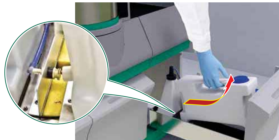
(removing of the water canister, mind the water canister / reservoir connection)
