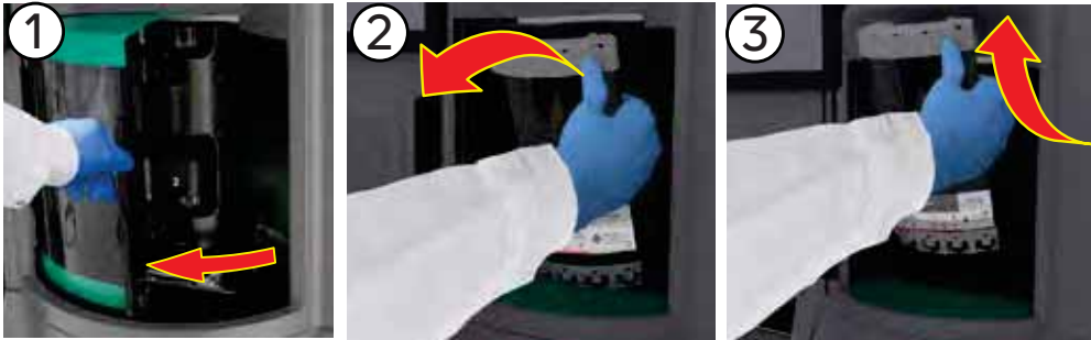
(magazine station door opening and magazine removing)
