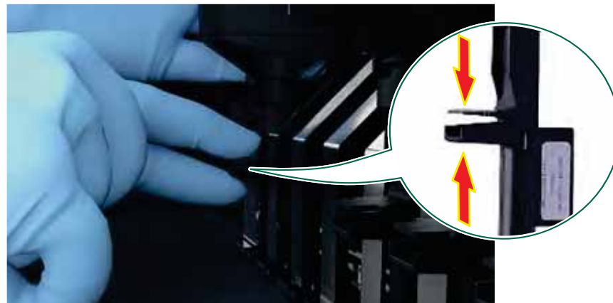
(reagent bottles lock mechanism)
