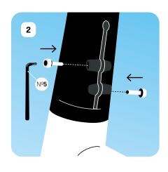
↑ Tighten the screws just enough to hold the handlebar in place. We'll be adjusting the height later on.
