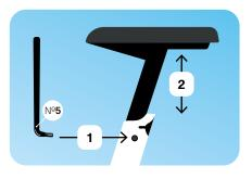
↑ Remove the rubber cap and loosen the screw. Slide the seat to your preferred height, tighten the screw, and put the rubber cap back on.
