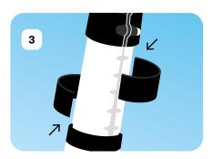
Place one or the two spacers, loosen the screw and slide the handlebar down.
