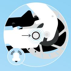
↑ Gently kick the Kick Lock button on the left side of the wheel. You'll hear a locking sound, that means the rear wheel is immobilized and the alarm is enabled.
