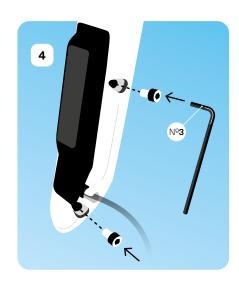
→ Tighten the two screws into the motor cable cover. Make sure both of them are secure.
