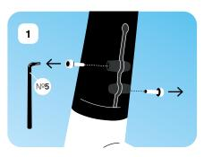
↑ Remove the two screws on the side.
