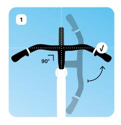
↑ Rotate the handlebar so that it forms a 90° angle with the bike frame.
