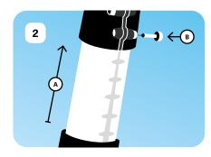
↑ Lift up the handlebar (A), then tighten one of the screws to keep it in position (B).
