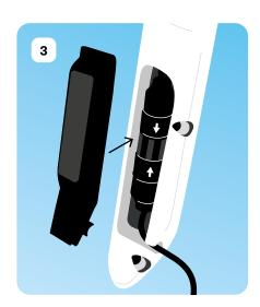
↑ Push the cable and connector into the fork leg and put the plastic cover over the motor cable notch on the front fork.
