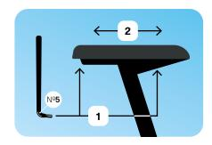
↑ Loosen both screws underneath the saddle, adjust the seat to your preferred position, and tighten the screws.
