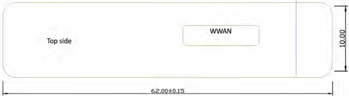
Fig.10 Antenna position of EUT
