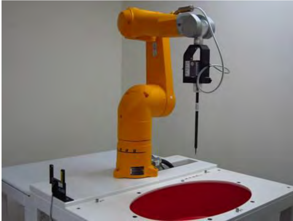
Fig.1 Photograph of the SAR measurement system
