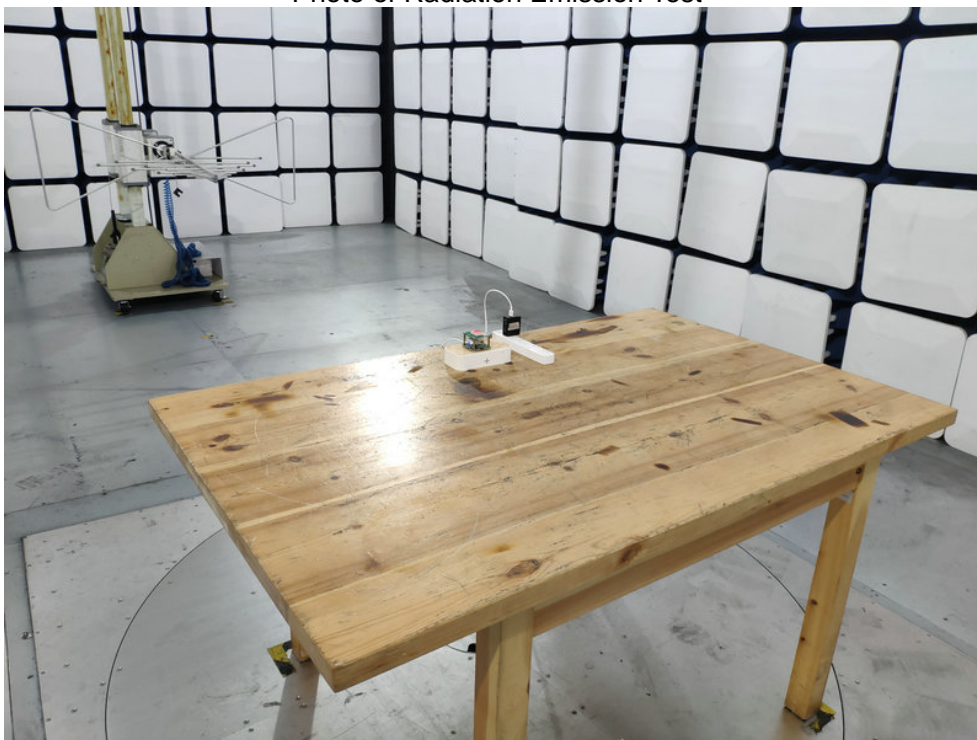
Photo of Radiation Emission Test
