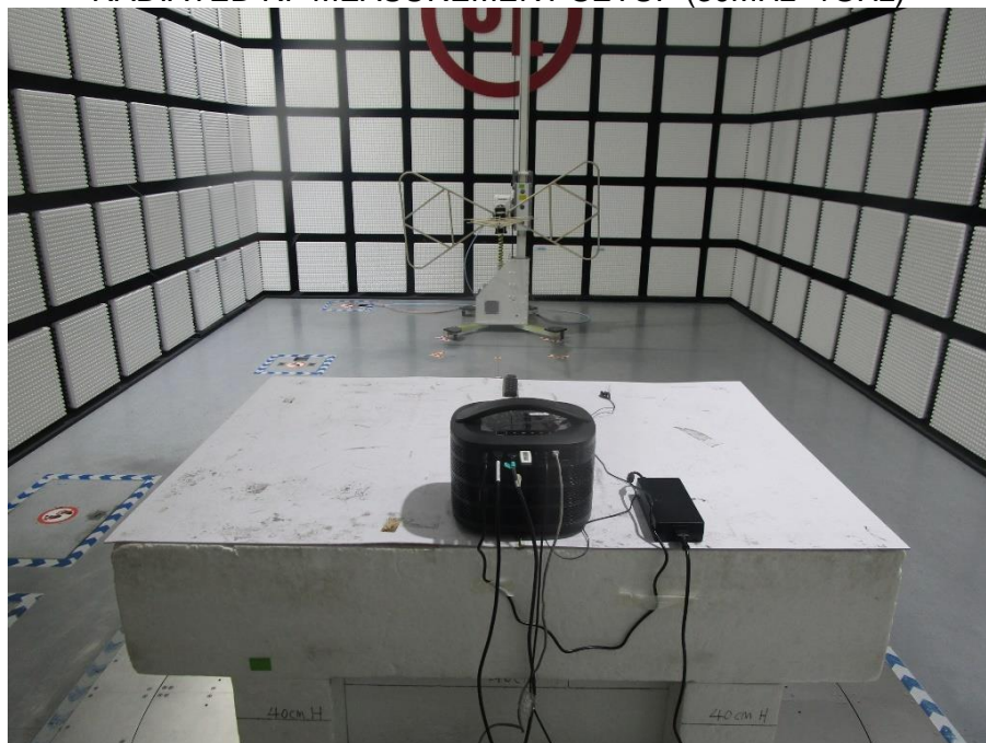
RADIATED RF MEASUREMENT SETUP (Below 30MHz)
