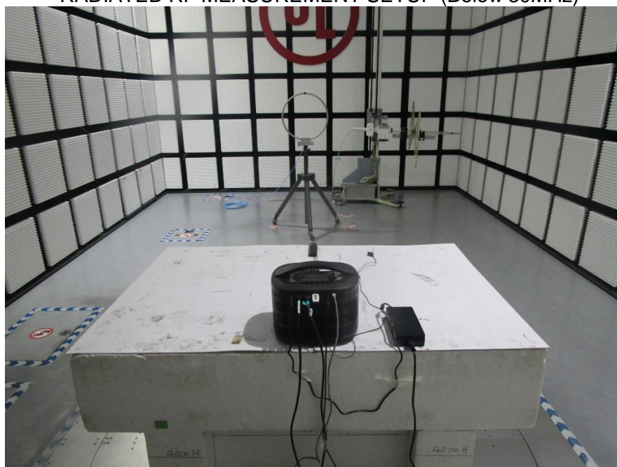
RADIATED RF MEASUREMENT SETUP (Below 30MHz)
