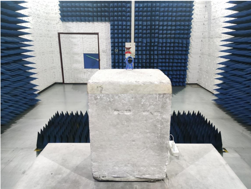
RADIATED EMISSION TEST SETUP ABOVE 1GHz
