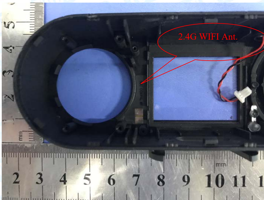
Photo 25 Internal of EUT
