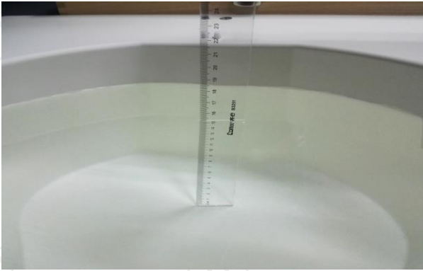
The Body Liquid of 2450MHz (15.3cm)
