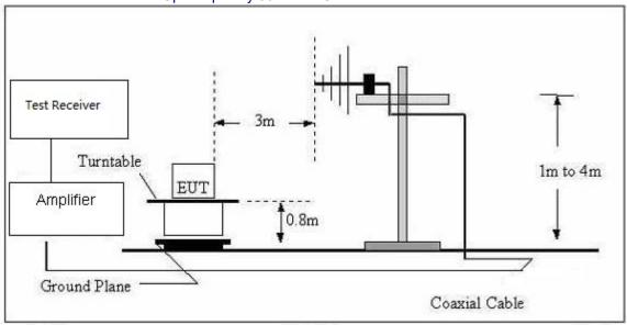
(C) Radiated Emission Test-Up Frequency Above 1GHz
