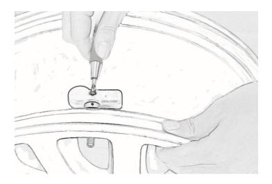
Step 3: Tighten the air nozzle fixing nut with a wrench to complete the installation. Note that the wrench uses a torque of  $7 \text{ N} \cdot \text{m}$ .
