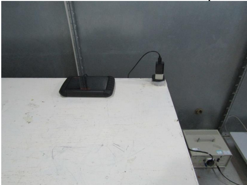
Measurement of Conducted Emission Test Set Up
