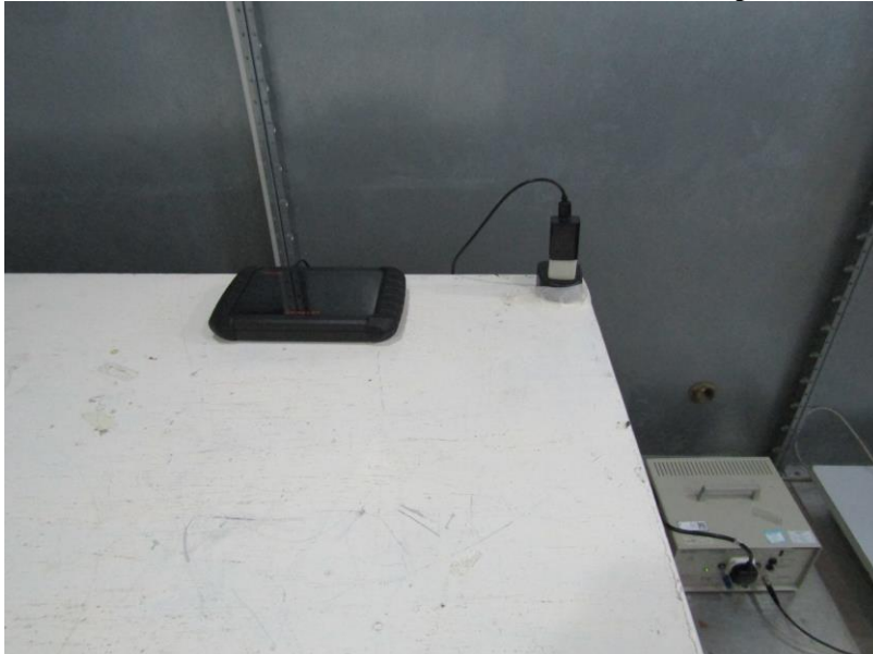
Measurement of Conducted Emission Test Set Up
