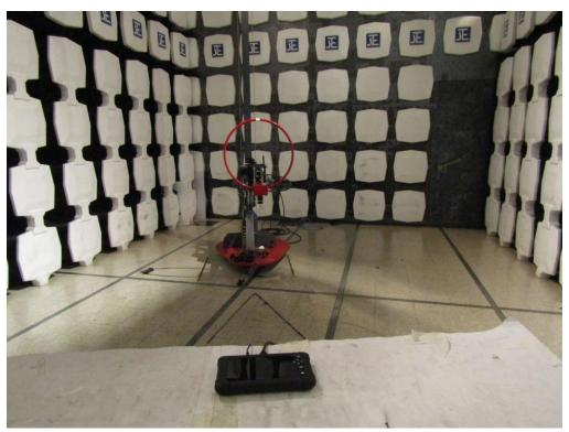
Measurement of Radiated Emission Test Set Up
