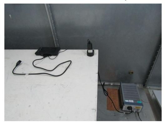
Measurement of Radiated Emission Test Set Up
