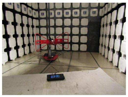
Measurement of Conducted Emission Test Set Up
