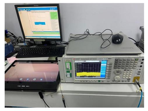
Conducted Emissions at AC Power Line (150kHz-30MHz)
