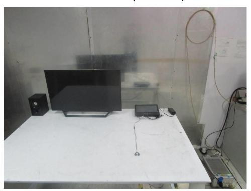
Radiated Emissions & Radiated Emissions which fall in the restricted bands
