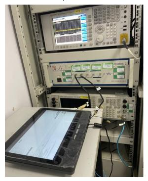
Conducted Emissions at AC Power Line (150kHz-30MHz)
