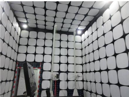
There is a holder to keep the RF antenna at the high 1.5 m above the floor.
