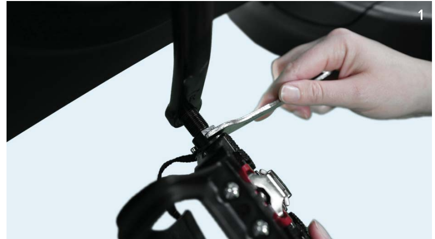
It is important to ensure pedals are installed properly and routinely tightened.
