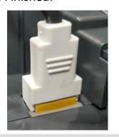
Note: if the 8pin cable assembling opposite, it will interfere with meter PCBA.
