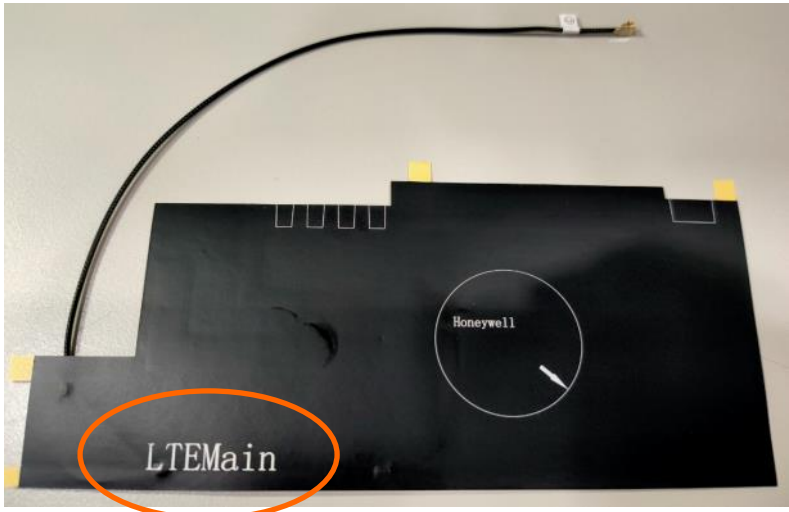
Antenna LTE Main _ No.3
