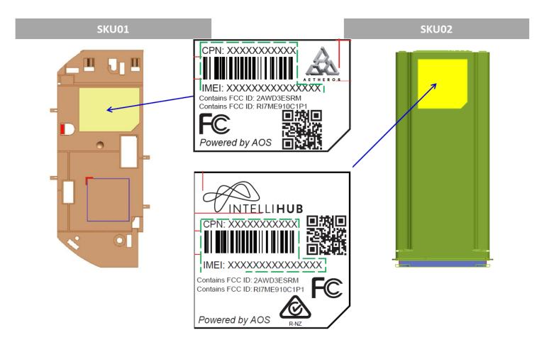
SKU1 is antenna housing included IoT Module & Electric meter So you can find the FCC label on the bottom side
