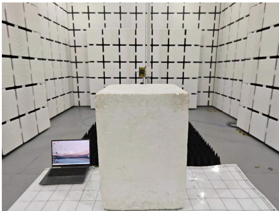
Set-up for Radiated Spurious Emission, Above 1GHz
