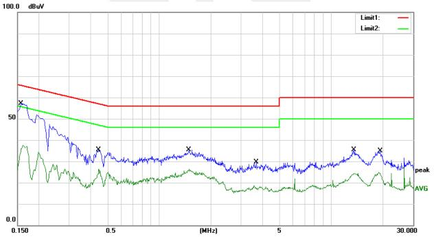
Note: The test voltage is 100-240V, both of which have assessment tests, and the worst test data is in the report.
