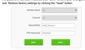
6. If you have made an incorrect setting adjustment or forgot the set password, you can restore factory settings on both transmitter and
