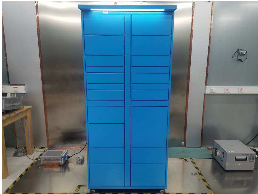
Photograph 3: Set-up photo for Conducted Emissions on AC Mains
