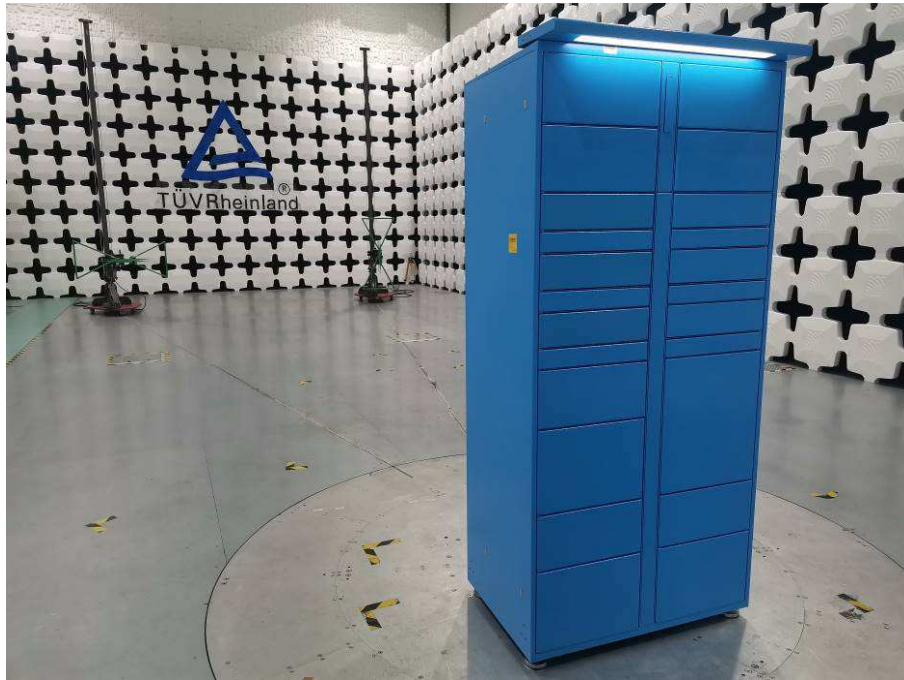
Photograph 1: Set-up photo for Radiated Emission, Below 1GHz
