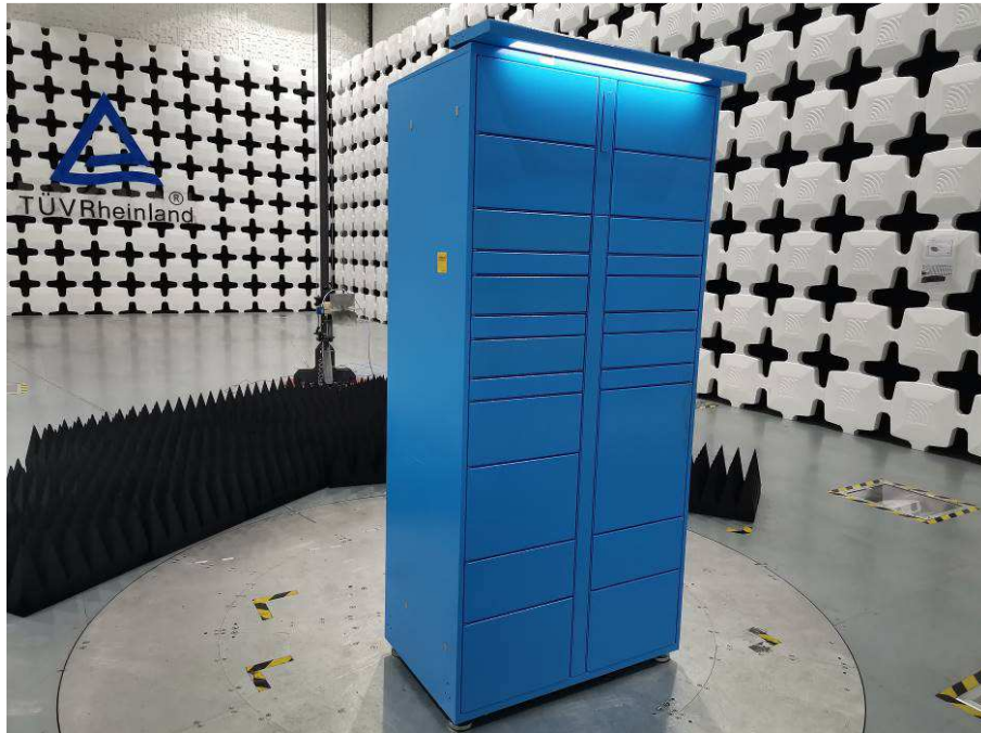
Photograph 2: Set-up photo for Radiated Emission, Above 1GHz
