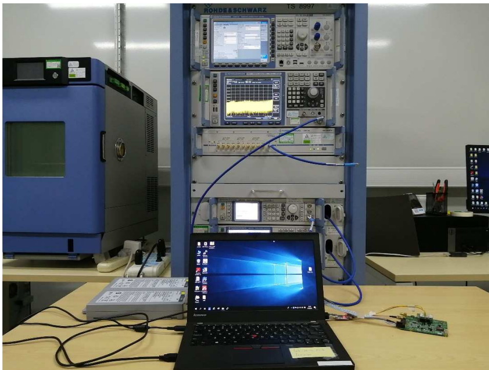
Photograph 2: Set-up for Conducted Measurements
