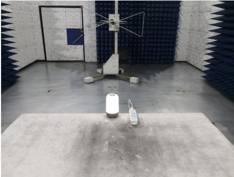
FCC RADIATED EMISSION TEST SETUP ABOVE 1GHZ
