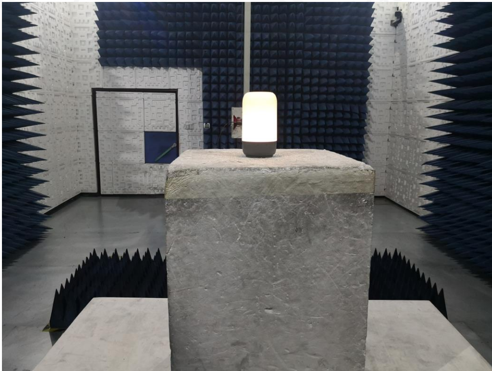
FCC RADIATED EMISSION TEST SETUP ABOVE 1GHZ
