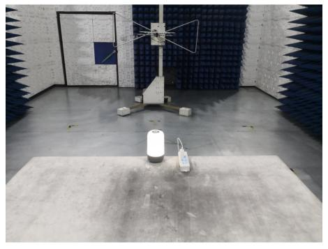
FCC RADIATED EMISSION TEST SETUP ABOVE 1GHz
