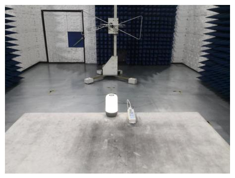
FCC RADIATED EMISSION TEST SETUP ABOVE 1GHZ
