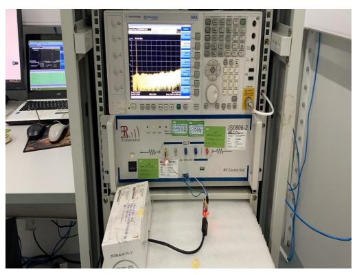
**ADAPTER-2** FCC RADIATED EMISSION TEST SETUP BELOW 1GHZ
