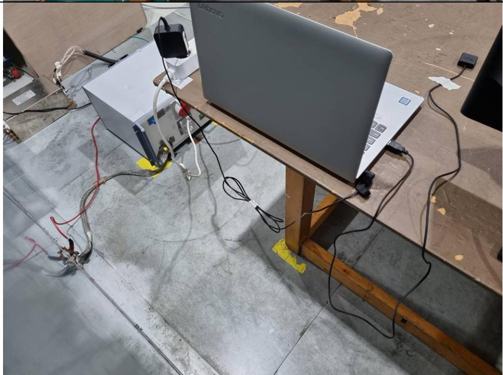
**Radiated Emission Test Set Up (Below 1 GHz)**
