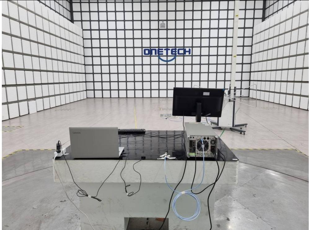
**Radiated Emission Test Set Up (Above 1 GHz)**
