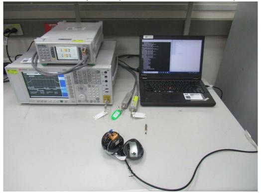
**Conducted Setup Photo (Measurement at Antenna Port)**
