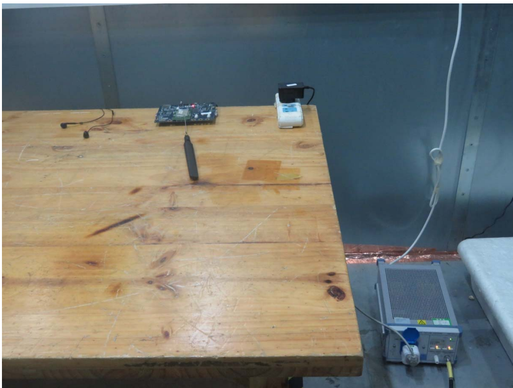
Picture 2 Conducted Emission Test Setup
