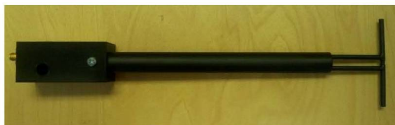
Figure 1 – MVG COMOSAR Validation Dipole
