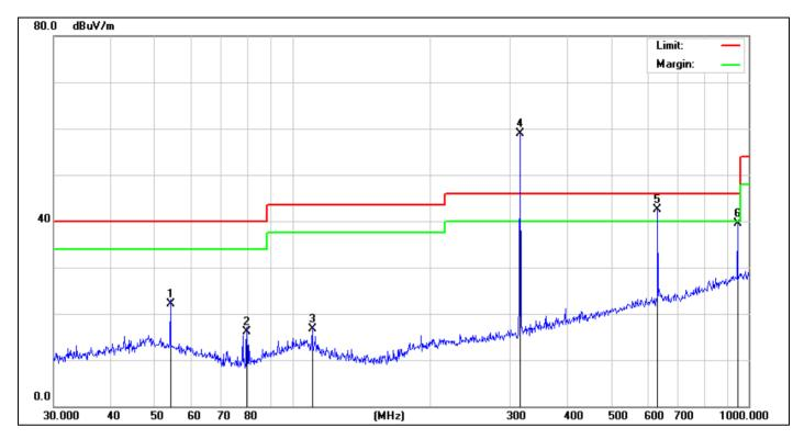
Site: LAB Antenna::Horizontal **Temperature(C):26(C)** Limit: FCC Part 15 C 3m Radiation **Humidity(%):60%** EUT: RF transmitter **Test Time:** 2021-04-26 M/N.: RT38A **Power Rating:** DC 3V TX**Test Engineer:** Mode: **Dyson** Note:
