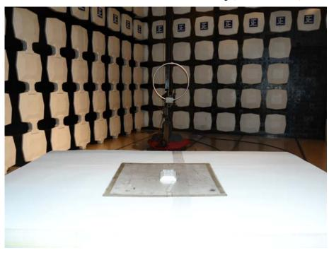
Measurement of Radiated Emission Test Set Up (30Hz – 1000MHz)
