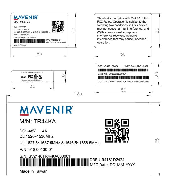
The label is made of PET self-adhesive; the glue material is pressure-sensitive adhesive, the main component is rubber or resin. The FCC IC label is permanently affixed on the device with an adhesive.
