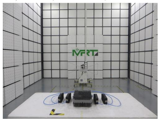
Description: Transmitter Spurious Emissions Test Setup Above 1GHz
