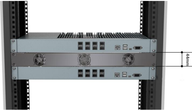
Figure 8. Separation of Adjacent A2
