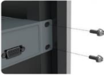
Figure 7. Fix A2 with Screws
