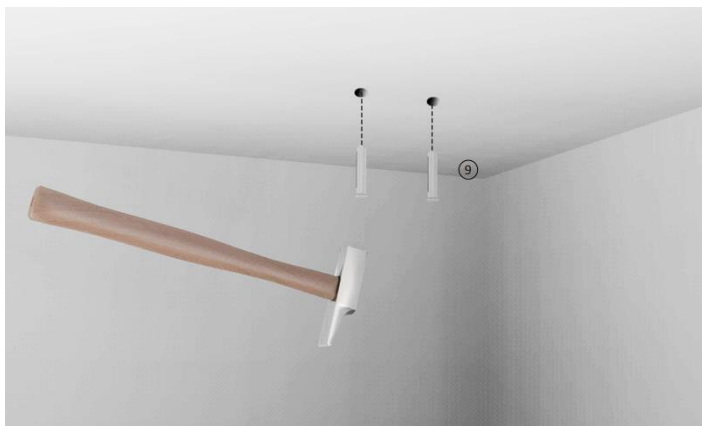
Figure 31. Insert Plastic Wall Plugs
