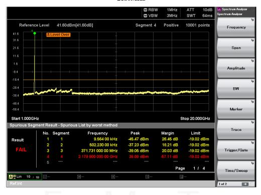
Note:- Marker in Segment 4 is desired intentional frequency of EUT, Hence, considered as PASS.
