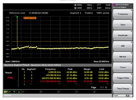
Note:- Marker in Segment 4 is desired intentional frequency of EUT, Hence, considered as PASS. 2150MHz
