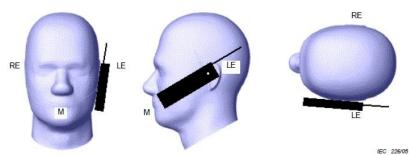
Cheek position of the wireless device on the left side of SAM
