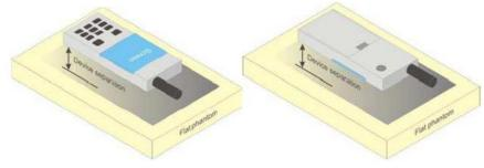
Test positions for body-worn devices
