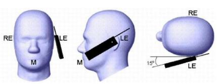
Tilt position of the wireless device on the left side of SAM
