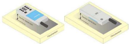
Test positions for body-worn devices
