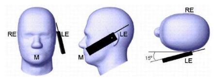
Tilt position of the wireless device on the left side of SAM
