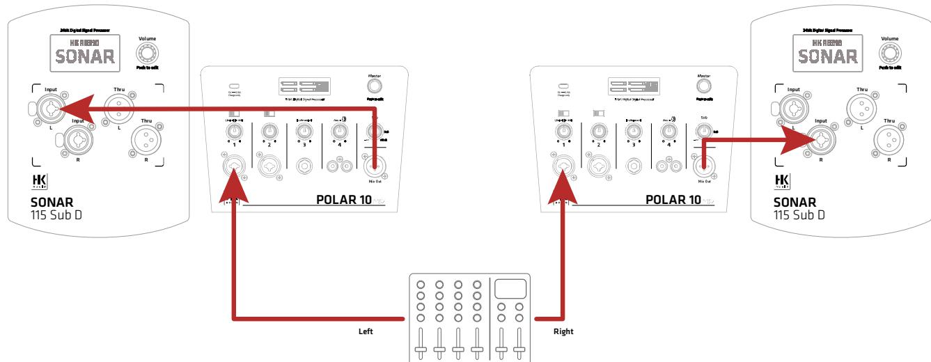
Sub extension for POLAR 10 MK2 & POLAR 12 MK2 with one SONAR 115 Sub D
