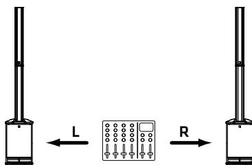
If you wish to run two POLAR 10 MK2 or POLAR 12 MK2 in stereo, route the mixing console's left channel to the system on the left and its right channel to the system on the right. Make sure the DSP settings for Mode, EQ, Delay, and so on are identical for both systems. See chapter 3 for more on this.
