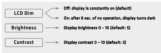
**LCD Dim:** Deactivate (Off) this function if you want the display to remain bright. Activate it (On), and the display will dim eight seconds after you last used the Master knob. The readout darkens, but it will remain clearly legible. As soon as you use the Master knob, the display will brighten to the set level.
