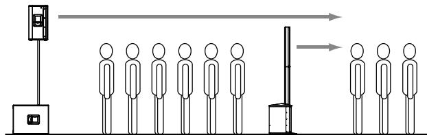
POLAR's Delay function lets you use it for a delay line. See section 3.2, Delay, to learn more about this. All you have to do is measure the distance between the main speaker and POLAR in meters, and enter that number to "Delay" in the DSP menu. POLAR factors the main speaker's delay into the equation, automatically calculates the delay time, and renders the signal with the proper delay.
