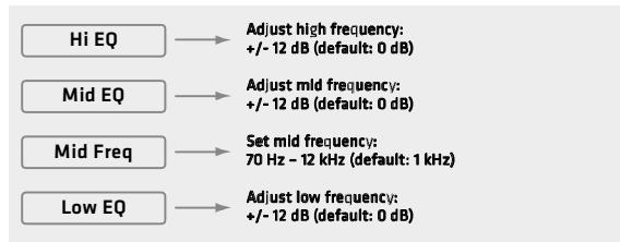
POLAR's three-band EQ serves to tune the system's overall sound. Hi EQ and Lo EQ are shelving filters; Mid EQ is semi-parametric.
