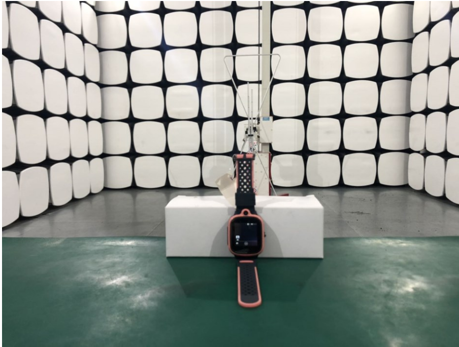
Radiated Emission test view (Frequency above 1GHz)
