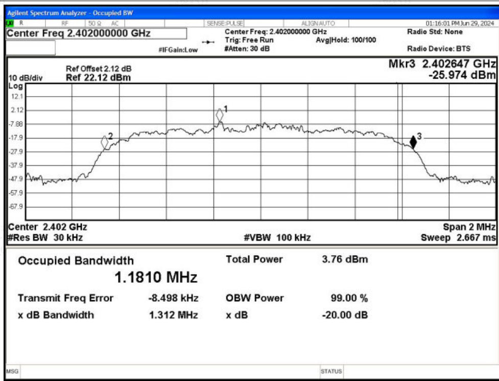
-20dB Bandwidth NVNT 2-DH5 2402MHz Ant1
