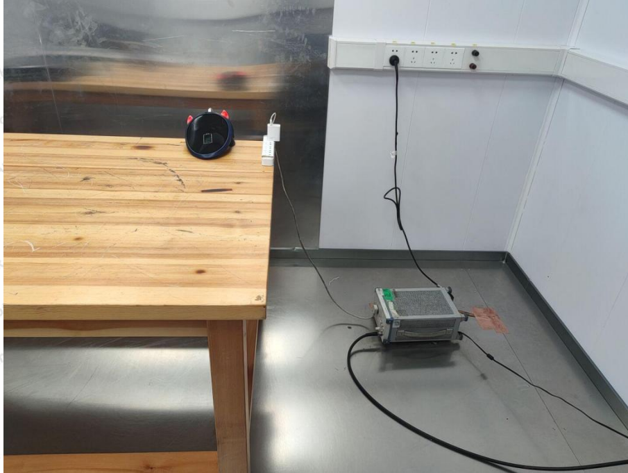
Conducted Emission at AC power line
